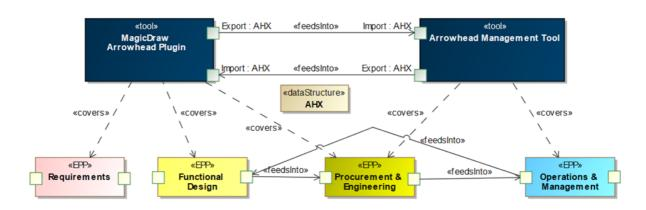
Here, in Task 4.2 and the present document, we focus on the <<dataStructure>>box called AHX in the middle. This is an example of a *toolchain interface*.
