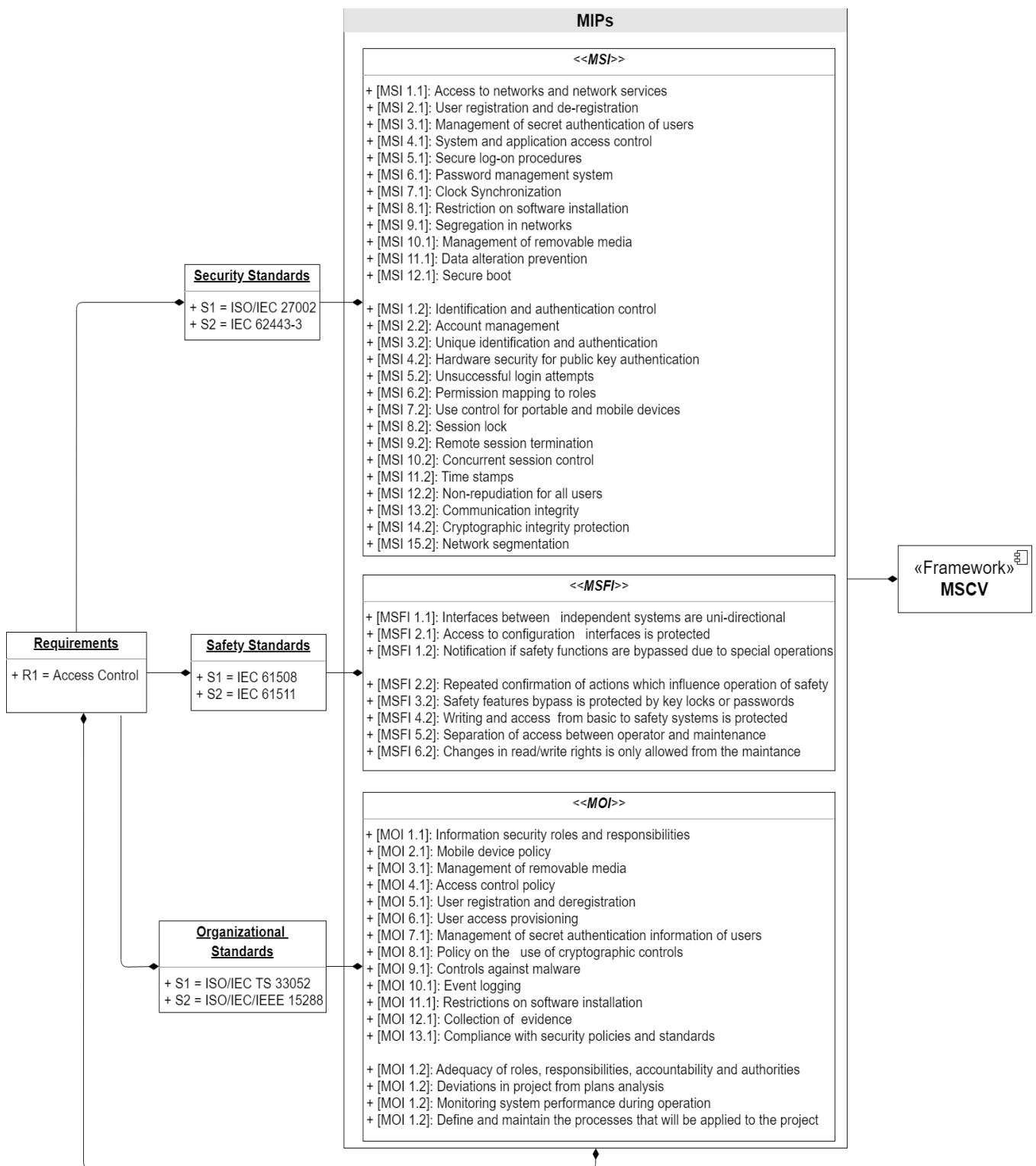
Figure 3. Example showing the usage of the metric model for security, safety and organizational standards considering the access control requirement
