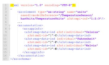
Fig. 7. Example of an annotated XML Schema with APPinfo
